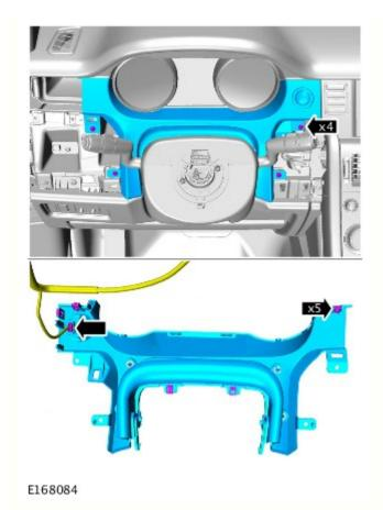
CAUTION: Extreme care must be taken when removing and installing the trim. Excessive force may result in damage to the component.
